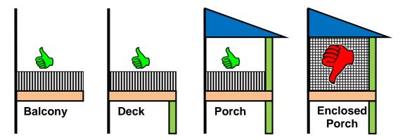
Composites are generally not designed for supporting loads. Column loads may not bear on composite decking.
