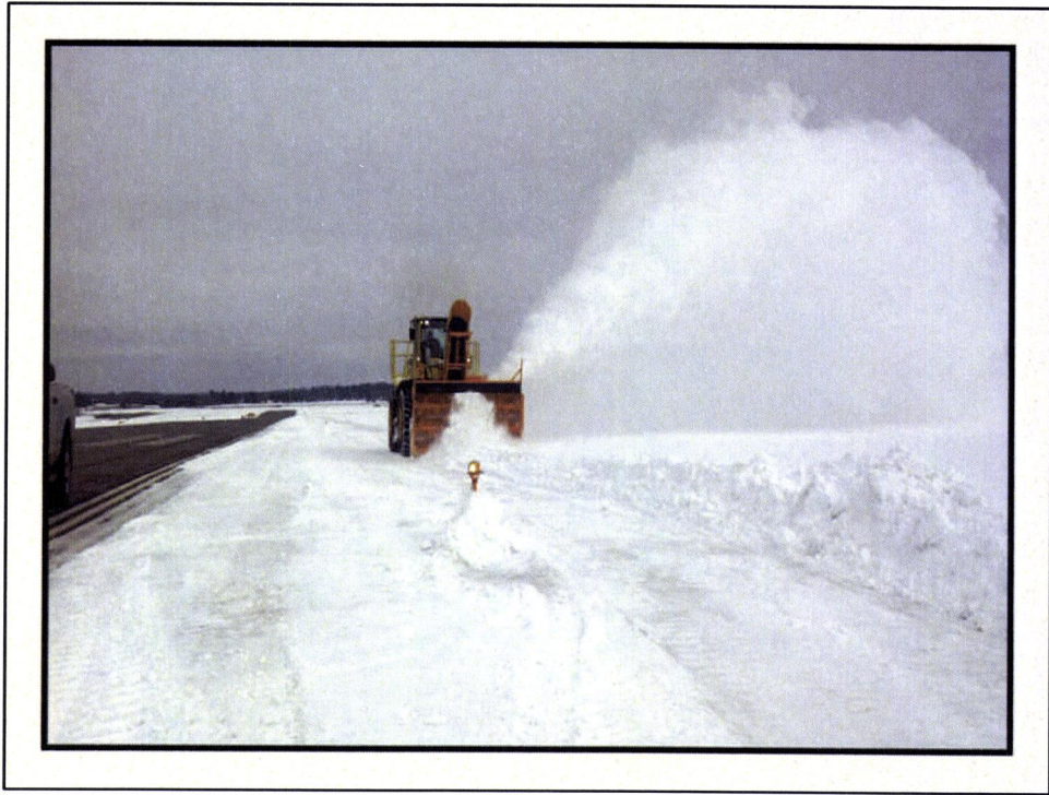
GR Itasca County Airport – Clearing Off Runway and Around Lights With Snowblower
